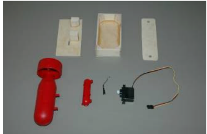
Parts of the bomb release. The clever bracket on the right was omitted to provide ground clearance.
