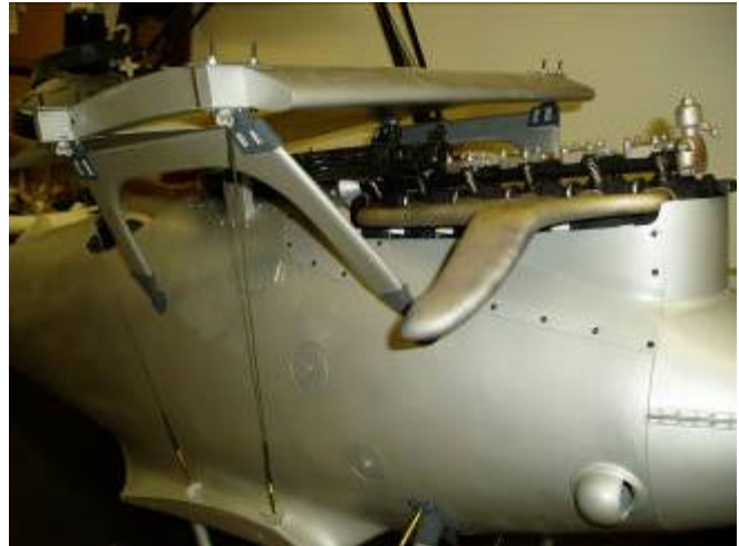
The front of the aircraft, showing scale engine, guns, and wing mounts.
