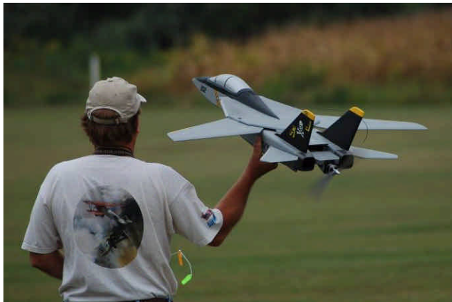
This electric F-14 had working swing wings that could be swept in flight.
