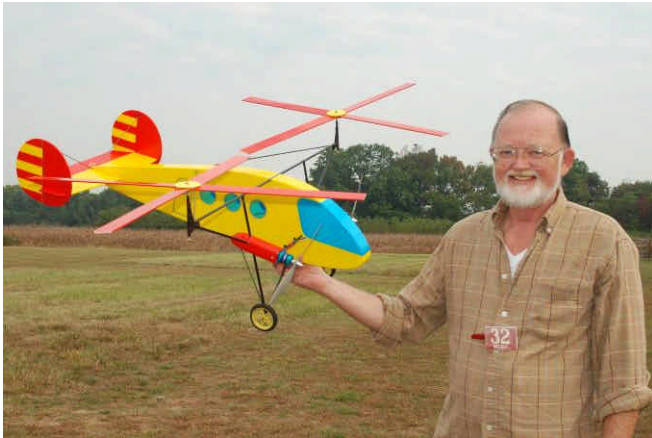
Dave Ramsey with his Gemini Twirl. Even the rotors are made from foam and carbon rods.
