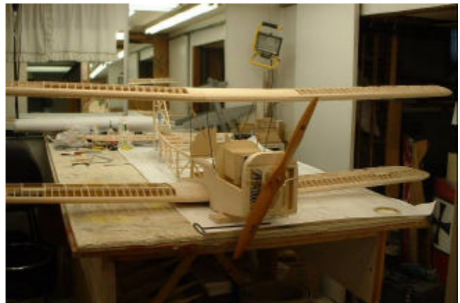
Fresh from Greg's factory, the framework of Keith Zimmerly's SE-5A sports a 3W50 gas engine.
