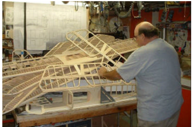
While some might shy from building atop a stack of wings, Greg says a few drops of CA here and there stabilize things nicely.
