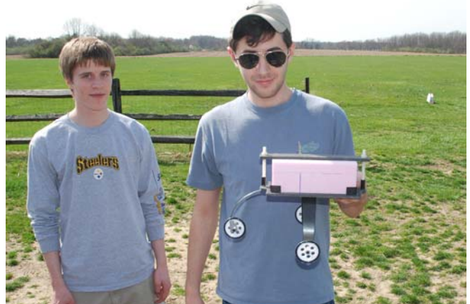
The electric model sported a detachable cargo bay mounted on the landing gear.
