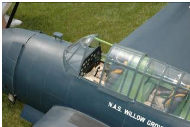
Detail started in the cockpit and included retracts, flaps, lights, a bomb-bay, and a bomb-drop.
